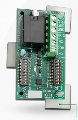
Trigger Current: -0.03 mA. @ 0V D.C., 0.9 mA. @ 12V D.C., 2.1 mA. @ 24V D.C., Operating Current: 8 mA. @ 12V D.C. (45 mA. with relay on), 10 mA. @ 24V D.C. (55 mA. with relay on), Operating Voltage: 10.5 - 28V D.C., Heavy duty 5 Amp. change over relay, 38mm x 72mm x 19.5mm (without feet), 50mm x 84mm x 23.5mm (with feet)
