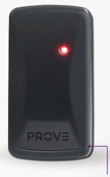
82.5mm x 43.7mm x 16.3mm Up to 10cm read range 50 mA. max, 8-28 Volts D.C. (Not compatible with pre existing Presco installations configured in Wiegand mode)
