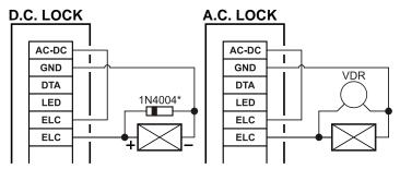
Use 1N4004 diode only when using a Door Strike, not a Magnetic Lock or Drop Bolt.
